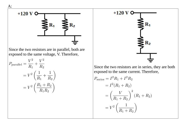
$$\frac{P_{\text{parallel}}}{P_{\text{series}}} = \frac{V^2 \left(\frac{R_1 + R_2}{R_1 R_2}\right)}{V^2 \left(\frac{1}{R_1 + R_2}\right)}$$
